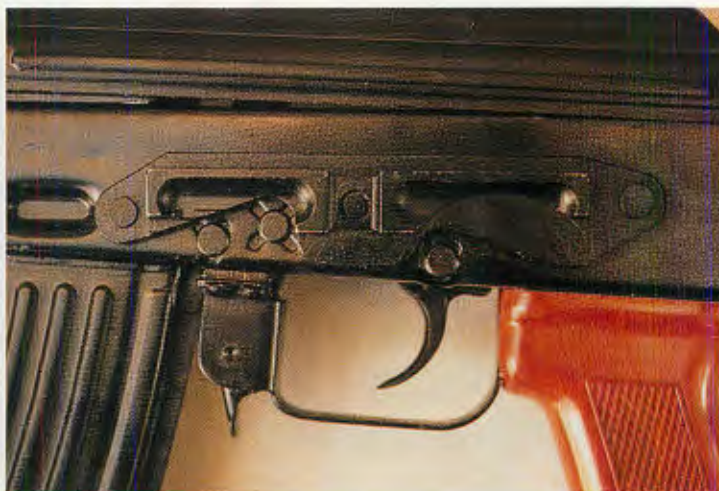
Romanian AKS-74 has a scope rail mounted to the left side of its stamped and riveted sheet-metal receiver.
